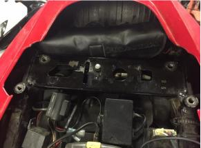
2. Install solo rack using the supplied hardware. The 35mm spacer should be used on the rear mounting holes along with the 50mm long bolts and washers.
