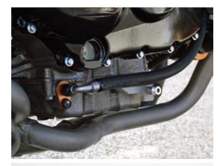
54. Install oil lines – longer hose (13" / 33cm) goes on the RH side, shorter hose (12.5" / 32cm) goes on the LH side
