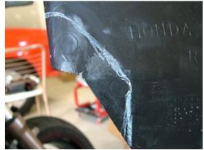
73. The first piece to be modified is the right-side inner plastic panel. It must be cut to clear the supercharger. About 1.25" (32mm) needs to be cut away from the portion that sits above & next to the supercharger.
