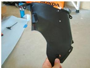
74. Next, you will need to modify the lower center fairing to clear the radiator. The best way to do this is to place the plastic in its correct location, but situated behind the radiator, and then using a grease pencil, crayon, or paint marker, trace around the radiator to mark where it needs clearance. Take the fairing back off and cut out the marked area.
